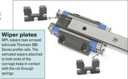
cation processes. The self-lubricating pieces also help bearings achieve their theoretical L10 lives. After about 30,000 km of travel, it is recommended that the self-lubricating wipers be replaced. However, this replacement is easily made onsite.
