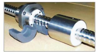
MPL inserts are used on Danaher Motion's selflubricating ball screws. Extruded, round bars are machined into a lubrication element contained in the ball nut.
