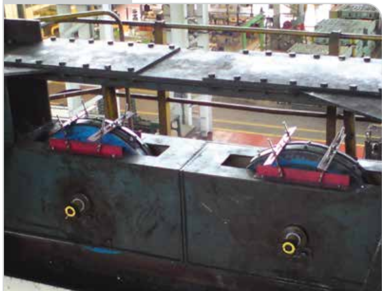
Two wheels in the crane fitted with the MPL flange lubrication system.
